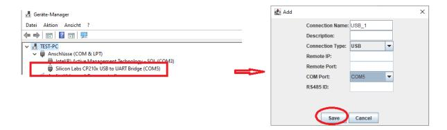
• Choose icon view or double-click the configured connection window to see the user interface of the appropriate power supply. You can manage several connections by using the Add/Edit/Delete buttons.
